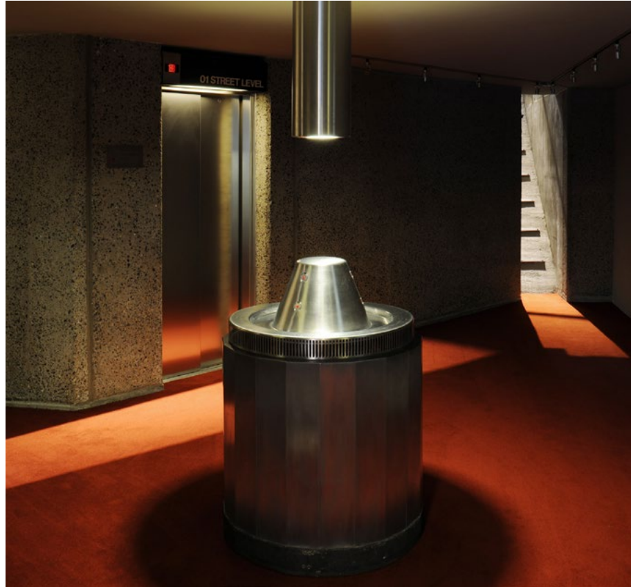
Lighting for lift doors + panel with daylight from escape stairs
